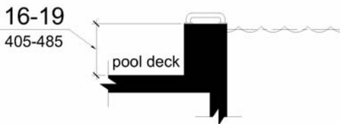
Fig. 75 Transfer Wall Height
